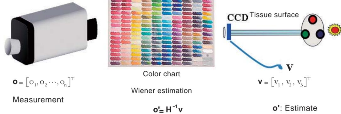
Figure 7. Measurement of the Spectral Reflectance by the Wiener Estimation.
